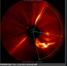
•StereoCat, a tool developed by the CCMC (Jack), allows one to derive parameters of a CME including its radial velocity, longitude, latitude, and opening angle.
